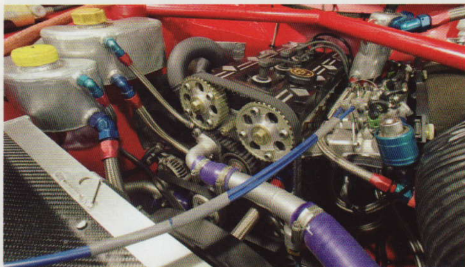
Colin's last MkII ran a big-spec 2-litre BDA; now he's gone for Millington power. These beauties roll out at 2.5-litres and run to 300+ bhp using natural aspiration...
