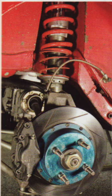
Turreted rear runs Proflex coil-overs, APs and a Sierra 7.5 inch diff.
